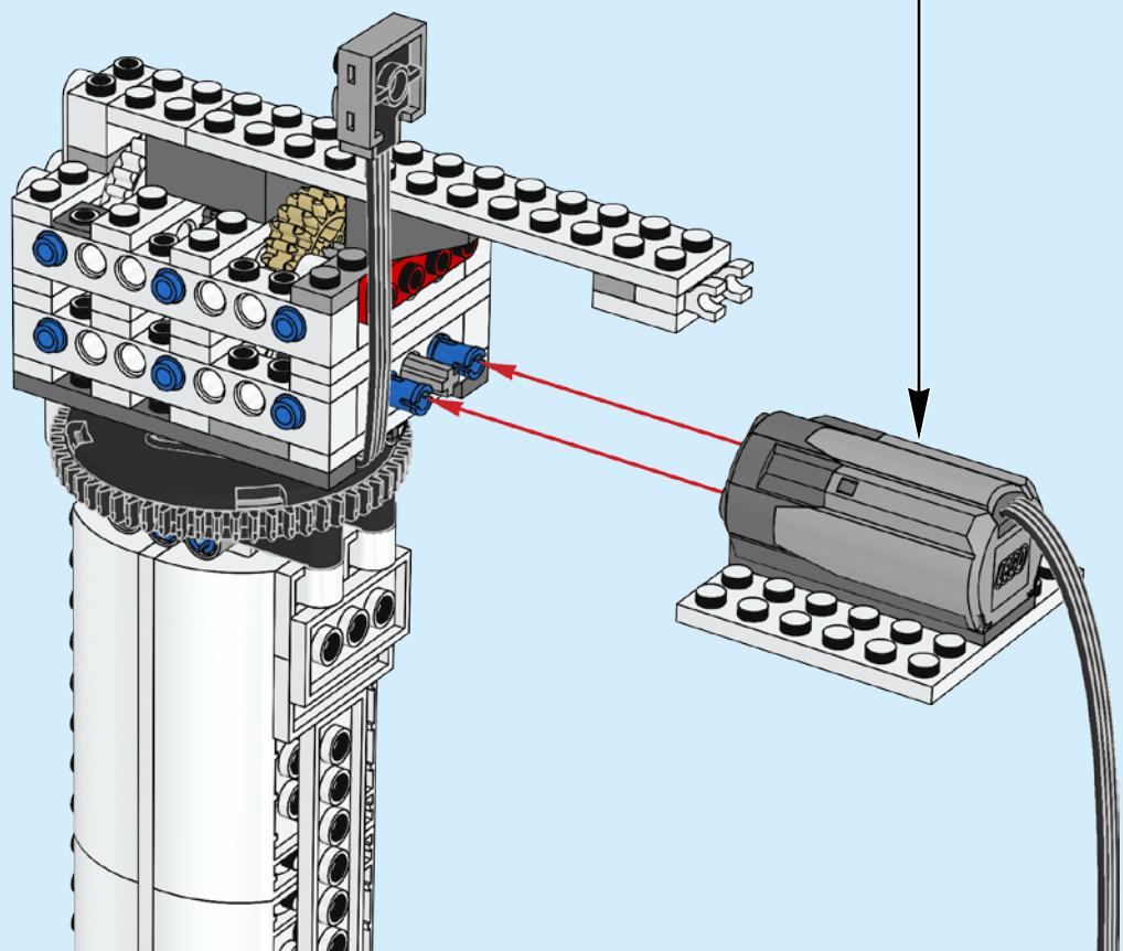
*The nacelle within the model contains a generator to convert the energy captured by the blades to electricity.*
